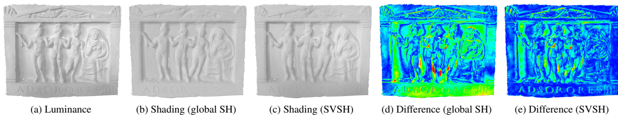
Figure 11. Estimated illumination of Relief dataset: the differences between input luminance (a) and estimated shading (b) and (c) are less for SVSH (e) than for global SH (d), meaning a better approximation of the illumination.
