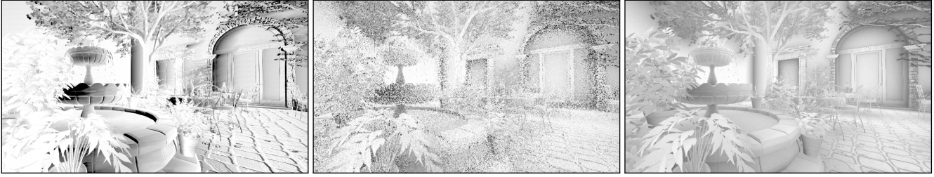
Figure 9: AO from 99 spiral taps ( left ) without rotation and a suboptimal \tau , ( center ) unbiased in 2D via pattern rotation, and ( right ) with \tau chosen using our screen-space QMC optimization. Results are shown without reconstruction to better illustrate the noise reduction.
