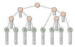
**Figure 2:** Ordered binary radix tree. Leaf nodes, numbered 0–7, store a set of 5-bit keys in lexicographical order, and the internal nodes represent their common prefixes. Each internal node covers a linear range of keys, which it partitions into two subranges according to their first differing bit.
