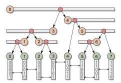
Figure 3: Our node layout for the tree of Figure 2. Each internal node has been assigned an index between 0–6, and aligned horizontally with a leaf node of the same index. The range of keys covered by each node is indicated by a horizontal bar, and the split position, corresponding to the first bit that differs between the keys, is indicated by a red circle.
