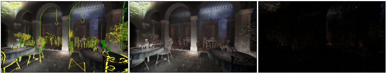
(a) Dark green: disocclusions filled by the second layer. Yellow: remaining disocclusions after considering both layers. (b) Indirect irradiance buffer E_i computed from (a). (c) Remaining error ( \times 5 ) in the indirect irradiance buffer E_i .
