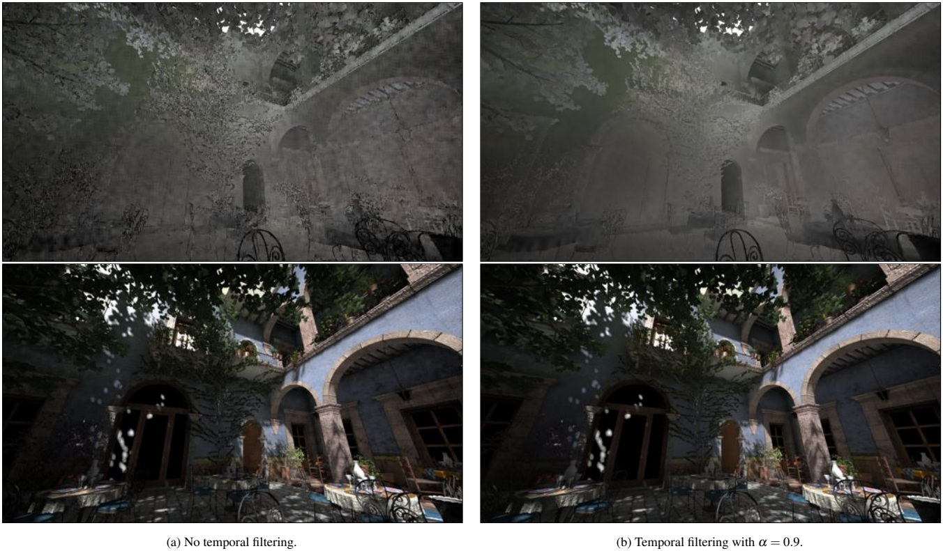
Figure 15: Temporal filtering smooths the noise due to undersampling in (a), producing the result in (b) without loss of spatial high-frequencies. The top row are the final indirect irradiance buffers, the bottom row are the final images. Both sets of images were produced with 3 taps per pixel per frame, with the taps randomly rotated each frame.
