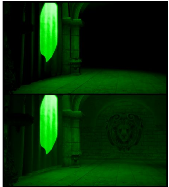
Figure 12: Top : 1-bounce radiosity ( p = 0 ) with a spotlight on the green banner in Sponza . Bottom : The converged result using p = 1 .
