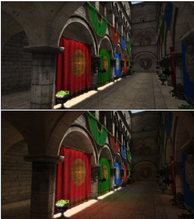
Figure 11: Top : Sponza with direct illumination and ambient occlusion of an environment probe, representative of typical real-time lighting today. Bottom : Replacing the environment light probe with screen-space radiosity brings out color bleeding and increases lighting contrast.
