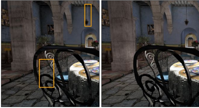
Figure 17: Animation frame from San Miguel in which the camera rapidly orbits the table. Left : \alpha = 0.98 creates ghosting artifacts due to reprojection error in temporal filtering. Right : \alpha = 0.9 reduces the ghosting artifacts. This value is still higher than we would recommend for most scenes.
