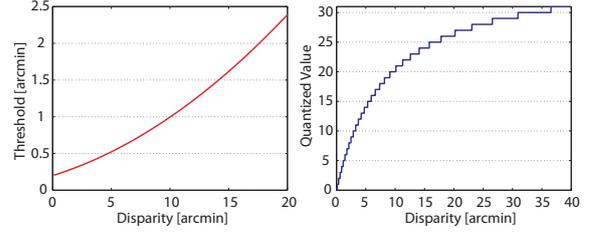
**Figure 1:** (left) *Threshold vs Disparity* function derived from [DRE\*11]. (right) *Example quantization levels of disparity response function for 5-bit encoding.*
