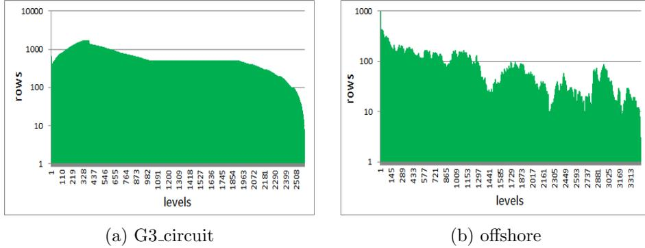
Figure 7: Distribution of rows into levels for level-scheduling approach `csrilu0`
