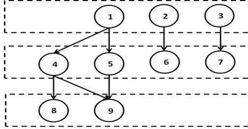
Figure 5: The data dependency DAG of the original matrix  $A$
