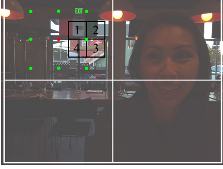
Figure 2: After dividing the reference image in tiles, our matcher looks at the center of each tile (red dot) and a set of predefined locations around it (green dots). It then computes a measure of cornerness based on the average luminance in the four quadrants around each candidate corner.
