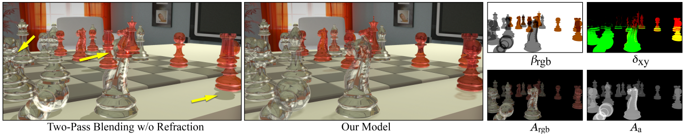
Figure 7: A glass chess set rendered with two draw calls and naive blending vs. our method in a single draw call for all transmissive surfaces. The \delta_{xy} term is visualized as RGB color ((\delta_x + 1)/2, (\delta_y + 1)/2, 0) . Arrows point to some errors in the naive rendering. Our result corrects the ordering and captures the phenomena of colored shadows with caustics, refraction, and colored transmission. © 2015 NVIDIA
