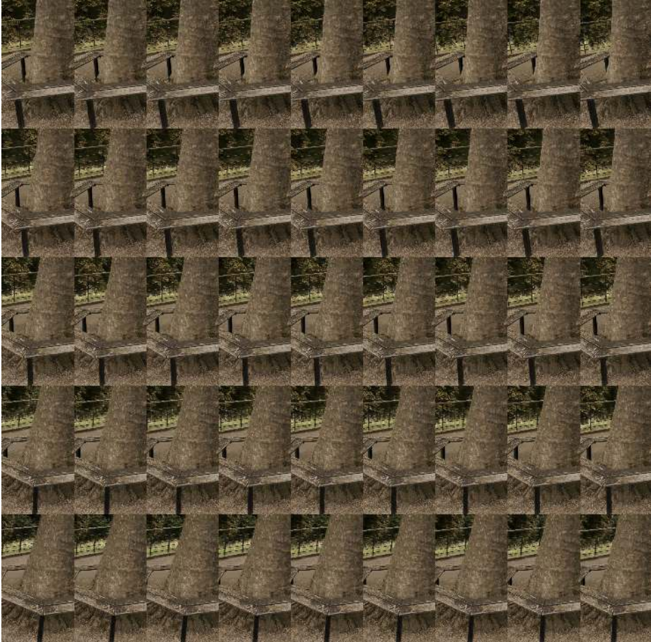
Fig. S15. Full 45-view light field quilt for TREEHILL scene from the MipNeRF-360 dataset [Barron et al. 2022] rendered using G2LF algorithm for Looking Glass Go display ( N_x = 512 , N_y = 910 , N_{\text{chunk}}=512 ).
