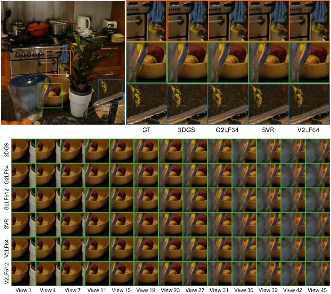
Fig. S3. Evaluation on the rendered COUNTER scene from the MipNeRF-360 dataset [Barron et al. 2022]. (Top) Visual comparisons between the ground truth, the baseline models, and our proposed methods. (Bottom) Rendered light field quilt views across horizontal viewpoints for different algorithms. Our methods preserve consistent multi-view appearance while trading off rendering quality and speed. The numbers appended to G2LF and V2LF denote the N_{\text{chunk}} .
