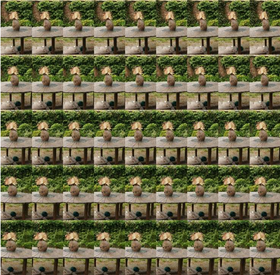
Fig. S7. Full 45-view light field quilt for GARDEN scene from the MipNeRF-360 dataset [Barron et al. 2022] rendered using G2LF algorithm for Looking Glass Go display ( N_x = 512 , N_y = 910 , N_{\text{chunk}}=512 ).
