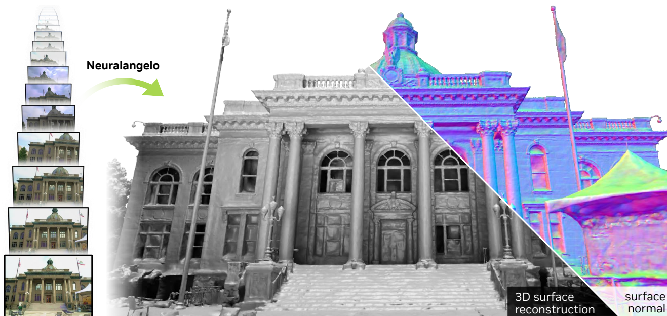
Figure 1. We present Neuralangelo , a framework for high-fidelity 3D surface reconstruction from RGB images using neural volume rendering, even without auxiliary data such as segmentation or depth. Shown in the figure is an extracted 3D mesh of a courthouse.
