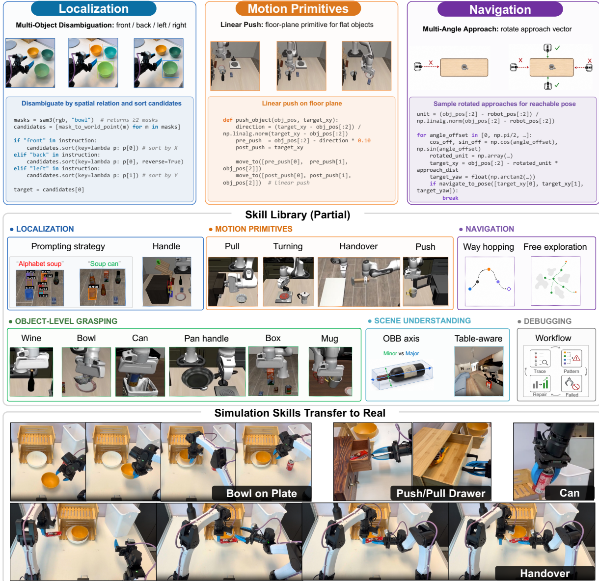
Figure 3: Skill library. ASPIRE stores validated, agent-discovered repair knowledge as reusable in-context skills rather than a fixed set of human-written primitives. Top: representative entries show learned skills about localization disambiguation, motion-primitive construction, and navigation recovery. Middle: the library grows across heterogeneous categories, including localization, navigation, motion primitives, object-level grasping, scene understanding, and debugging workflows. Bottom: selected skills discovered in sim are used as in-context guidance for real-robot programming, providing evidence that skills can transfer across embodiments. Additional skill examples and prompts are shown in Appendix A.
