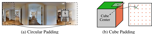
Figure 4. (a) We pad a side of the ERP by replicating pixel values from the opposite side. (b) We pad the green cube face with the interpolated value of the green point projected on to the orange face. Transparent squares indicate the convolution filters.
