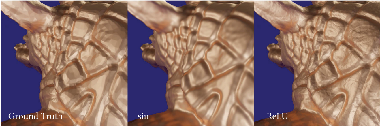
Fig. 18. Comparison of the effect of sin (middle column) and ReLU activation functions (right-most column) for the Armadillo example. The ground truth model (left) has both smooth geometry as well as flat surfaces from the coarse input mesh. The sin activation function tends to smooth out the sharp edges while ReLU can introduce more high-frequency noise.
