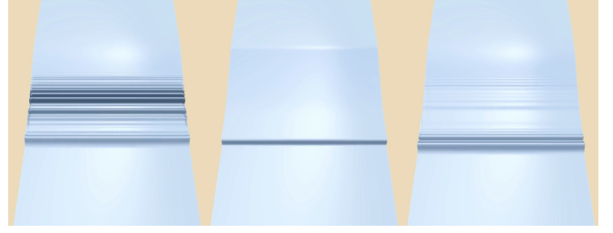
Fig. 5. Gradient penalty evaluation. This example started with an extremely steep wave (a step-function). Without the gradient penalty term in Equation 13 (left), the surface explodes into a large number of steep high-frequency surface waves. Enabling that term (right) gives results that look more like a SWE simulation (center) with enriched details.
