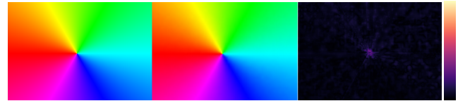
Fig. 19. A colorful and (presumably) difficult gradient texture compressed with NTC 0.2 does not show visible banding, color posterization, or discoloration. Left: Reference. Middle: Compressed. Right: FLIP error image and corresponding color map.
