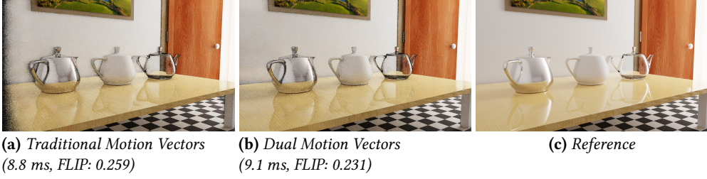
Fig. 6. Applying dual motion vectors [Zeng et al. 2021] provides a dramatic reduction of disocclusion noise which is severe in the VEACH AJAR due to undersampling. The result contains some correlated noise but does not show "copy-pasting" artifacts.
