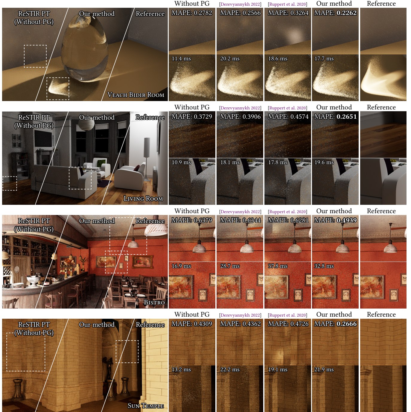
Fig. 5. Comparisons between ReSTIR PT without path guiding (Without PG), ReSTIR PT integrated with prior path guiding methods [Derevyannykh 2022; Ruppert et al. 2020], and our method. Note that all methods are evaluated with ReSTIR PT enabled and rendered with 1 spp. Our method produces cleaner results with lower noise and fewer correlation artifacts. In all comparisons, our method achieves the lowest MAPE.
