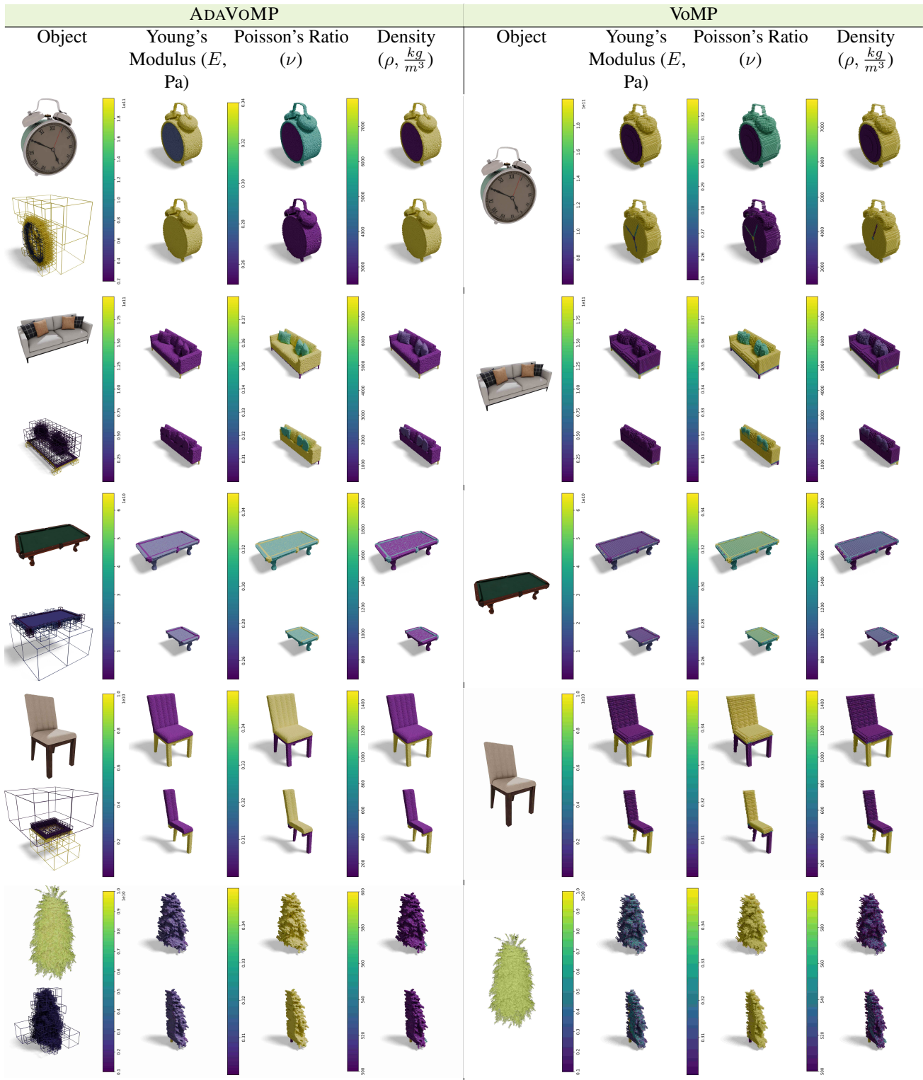
Figure 13. Inferred Mechanical Property Fields. We show additional mechanical property fields and slice planes through mechanical property fields estimated by ADAVOMP.
