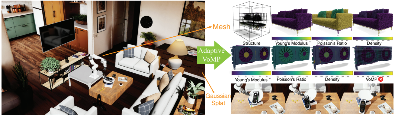
Figure 1. ADAVOMP generates high-resolution physically accurate volumetric mechanical property fields with detailed parts across 3D representations, enabling their use in building realistic interactive worlds and deformable simulations. We simulate a robot interacting with a high-resolution GPU and the sofa or pillows being stable under gravity in this Gaussian splat + mesh environment. (📺: 01:13)
