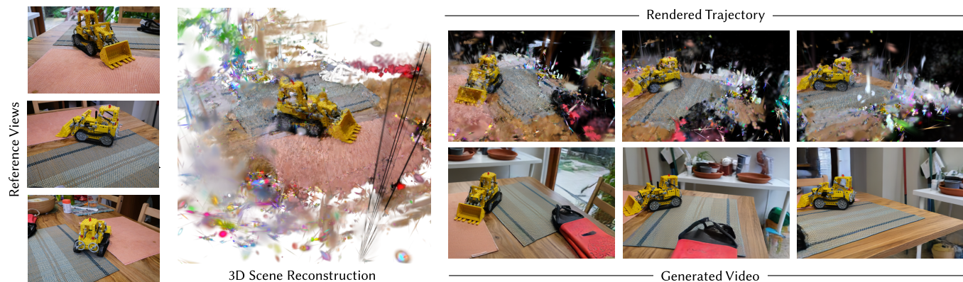
Fig. 1. ARTIFIXER enhances and extends existing 3D reconstructions in a highly efficient and scalable manner. Given an initial reconstruction, set of reference views, and an optional text prompt, it auto-regressively generates novel content that maintains a high degree of consistency with existing observations. ARTIFIXER can directly produce hundreds of novel views in a single inference pass or serve as pseudo-supervision to improve the underlying 3D reconstruction.
