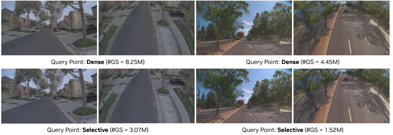
Figure 6: Query-point selection. Comparison of the Dense and Selective query-point strategies. The Selective strategy produces far fewer Gaussians (#GS) while maintaining comparable reconstruction quality.
