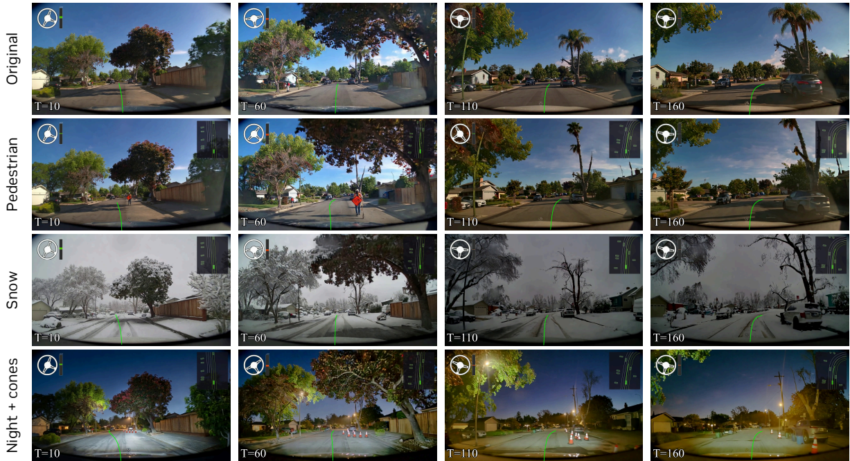
Figure 10: Controllable scenario editing. Starting from a given scene, OmniDreams supports targeted edits by modifying its conditioning inputs: text prompts can be used to modify appearance attributes such as weather and time of day of the first frame condition, and by also adapting the abstract world-scenario map, and ego-state conditioning changes the driven trajectory. Unedited attributes such as road geometry and distant scene context remain visually stable across variants.
