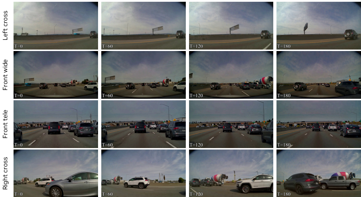
Figure 8: Multi-view generation. OmniDreams generates synchronized observations for multiple camera views from a shared scene state. Across cross-left, front-wide, front-tele, and cross-right cameras, road layout, dynamic actors, lighting, and scene context remain coherent over time, enabling closed-loop policies that consume multi-view camera inputs.
