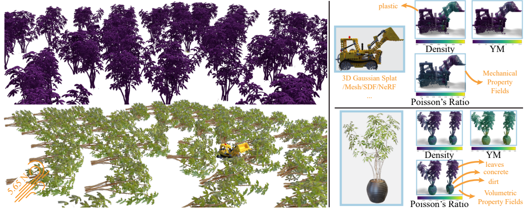
(e) Simulating Gaussian Splats at scale: an elastodynamic simulation of a Gaussian Splat bulldozer going through a forest of 100 Gaussian splat ficuses in the presence of wind; all materials predicted by VoMP (📺: 3:00).
