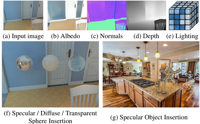
Figure 1: From a single image, our model jointly estimates albedo, normals, depth, and the HDR lighting volume. Key to our method is inferring continuous HDR 3D spatially-varying lighting, which is critical in producing high quality virtual object insertion with realistic cast shadows and angular high-frequency details.
