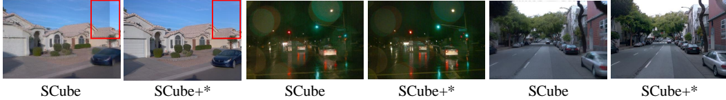
Figure 9: SCube+* . Results from the postprocessing network without per-scene optimization. White-balance inconsistencies from different views (marked in red box) can be fixed.
