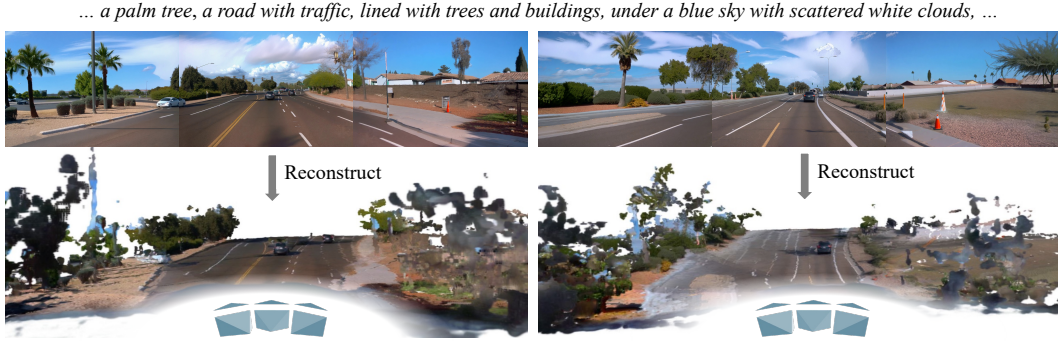
Figure 7: Text-2-Scene Generation. Given a text prompt, we could generate various multi-view images and lift them to 3D scenes with SCube. See Appendix D.3 for more text-2-scene results.
