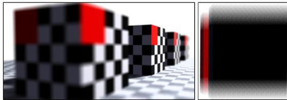
**Figure 5:** Stochastic rasterization images showing (a) correct defocus blur and (b) correct motion blur (two rising boxes). Post-process techniques are challenged by surfaces revealed by rotation, disocclusion, or defocus, because color and velocity information are missing.
