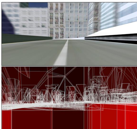
**Figure 10:** Top: our stress test for our  $z = 0$  algorithm includes very large triangles under large relative motion, which frequently triggers the case. Bottom: visualization of overdraw that shows moving triangles are worse, but not substantially worse, than static triangles. The camera for this image is centimeters above the poorly-tessellated area shown on the lower right in Figure 4.
