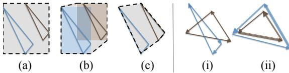
**Figure 3:** Some choices for bounding geometry. We use the 2D convex hull (c) because the cost of computing this tight bound is repaid in the per-fragment threads that are conserved. Note that the triangles may have arbitrary orientation with respect to each other, such as (i) or (ii).
