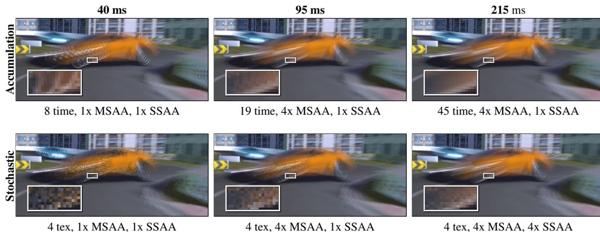
**Figure 9:** Comparison of accumulation buffering and stochastic rasterization for the same render times. Accumulation buffering renders a number of discrete ghosts equal to the number of time samples; stochastic rasterization creates noise. Insets are zoomed 5x. Images are cropped and downsized for printing from the full  $1920 \times 1080$  results; see our web page for the original data.
