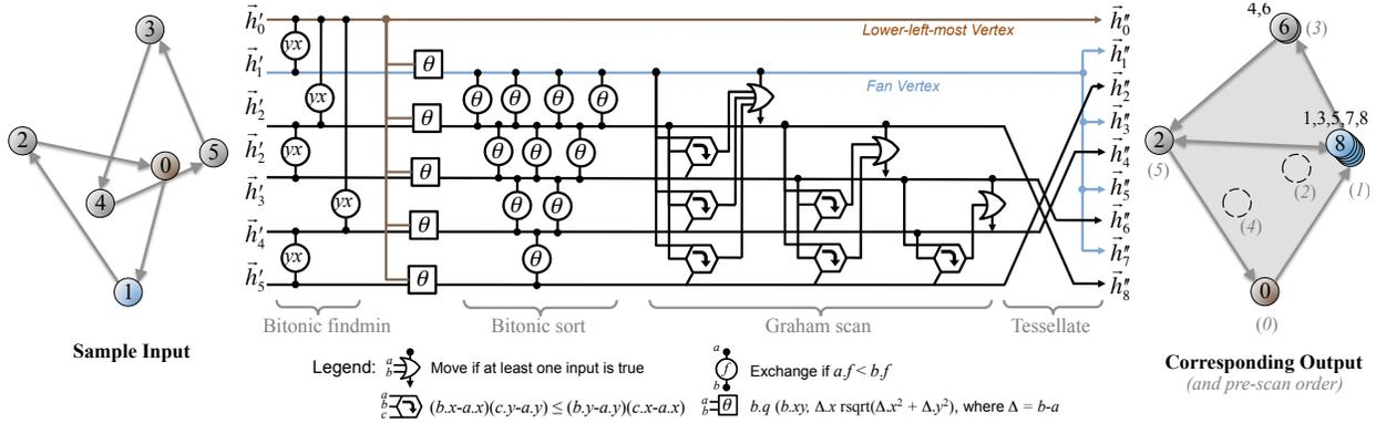
**Figure 2:** Our bounding geometry algorithm. The six screen-space vertices of a time-continuous triangle enter on the left in any order. Vertices forming the tessellation of the 2D convex hull exit on the right in triangle-strip order.
