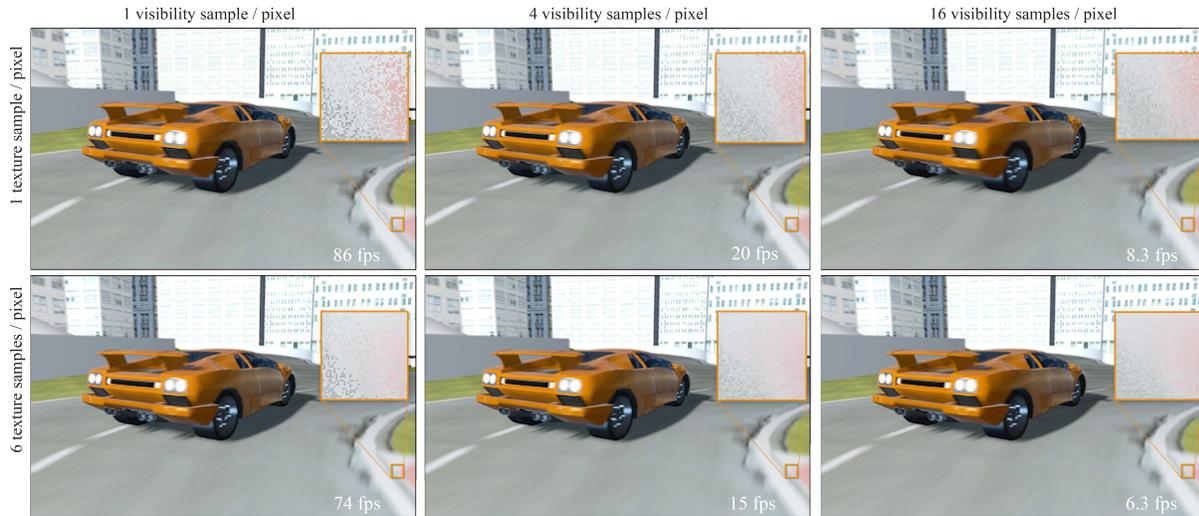
**Figure 7:** 130ktri racing scene with camera and object motion, rendered with motion blur. Along rows: Increasing texture filter size by the amount of motion or defocus provides improves sampling at texture edges, such between the red and white stripes in the 10x zoom insets. Along columns: Increasing visibility samples improves noise everywhere, including the geometric edge against the gray road on the lower-left of the insets, but at higher cost.
