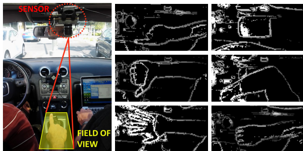
Figure 1. We modify an HDR, binary contrast sensor to enable the extraction of gray-level information. We then use this information to detect gestures in a car’s cockpit. The setup for the proposed system is shown in the left column. The center column shows three typical gestures (see Sec. 4). The rightmost column shows backgrounds, where the hand is either making a fist or is absent altogether.
