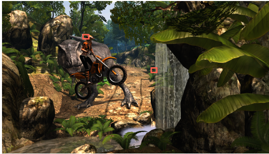
Figure 1: An ACAA frame, with close-ups comparing (a) Single-sampled image. (b) 8x ACAA image. (c) 8x MSAA image. ACAA renders opaque surfaces nearly identically to MSAA but uses half the framebuffer memory. Scene courtesy of Kishonti Informatics.
