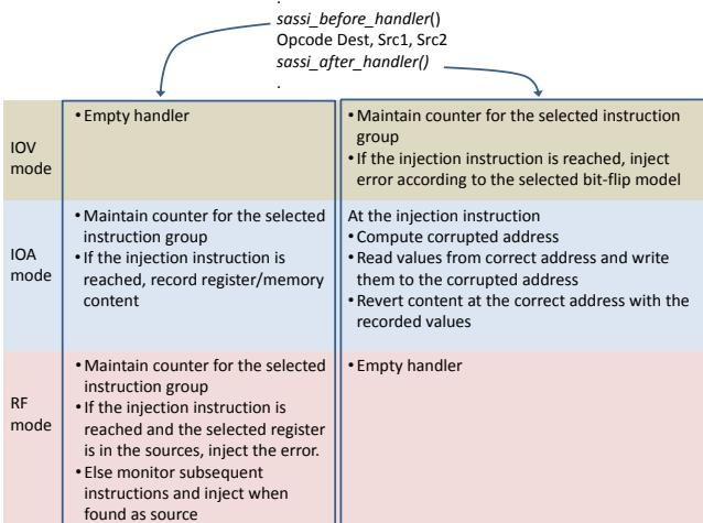
Figure 3: Error injection handlers for different modes.
