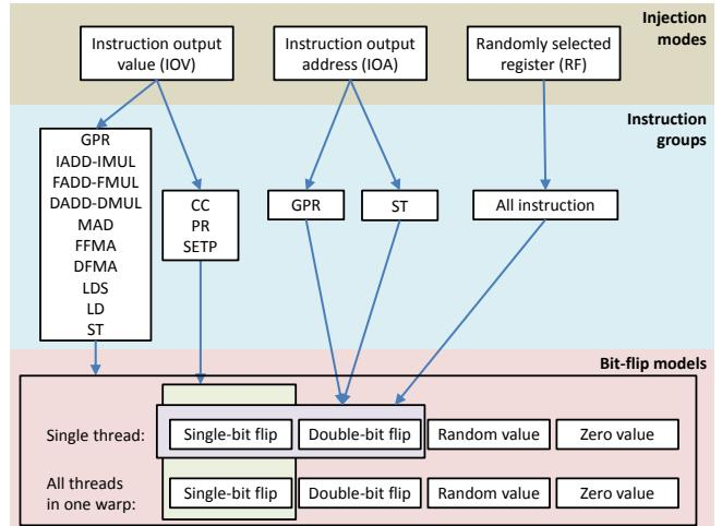
Figure 2: Summary of different error injection modes, instruction groups, and bit-flip models that SASSIFI provides.
