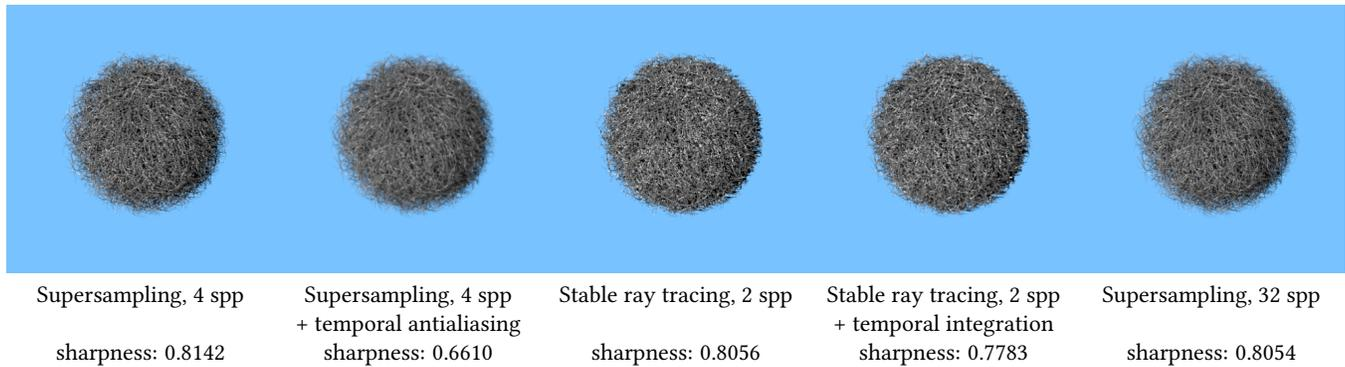
**Figure 5: Comparison of frames rendered for the hairball video. For each technique, we report the number of samples per pixel (spp) and the CPBD-based image sharpness. Stable ray tracing strikes a compromise between sharpness and temporal stability at the price of added spatial aliasing.**
