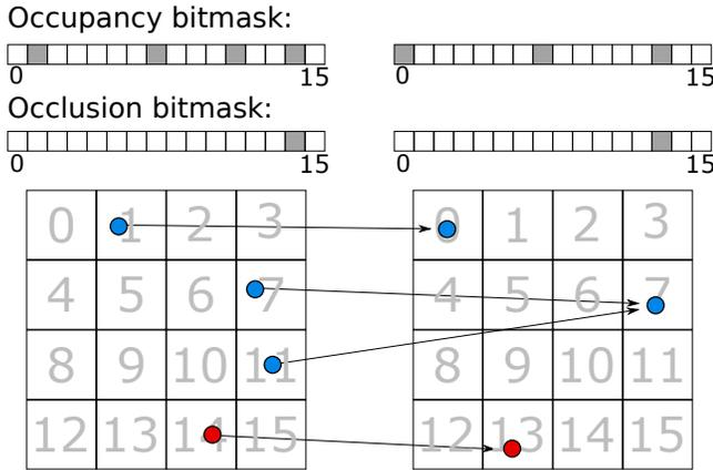
**Figure 3: Reprojection phase for an  $M=4$  set of subpixels from one frame, left, to the next, right, and evolution of the bitmaps. Both occluded and unoccluded samples are recorded in the occupancy bitmask. Occluded samples (red) also have a bit set in the occlusion bitmask. In the case of a collision between two samples (subpixel 7, right), the first unoccluded sample written to the subpixel is kept.**
