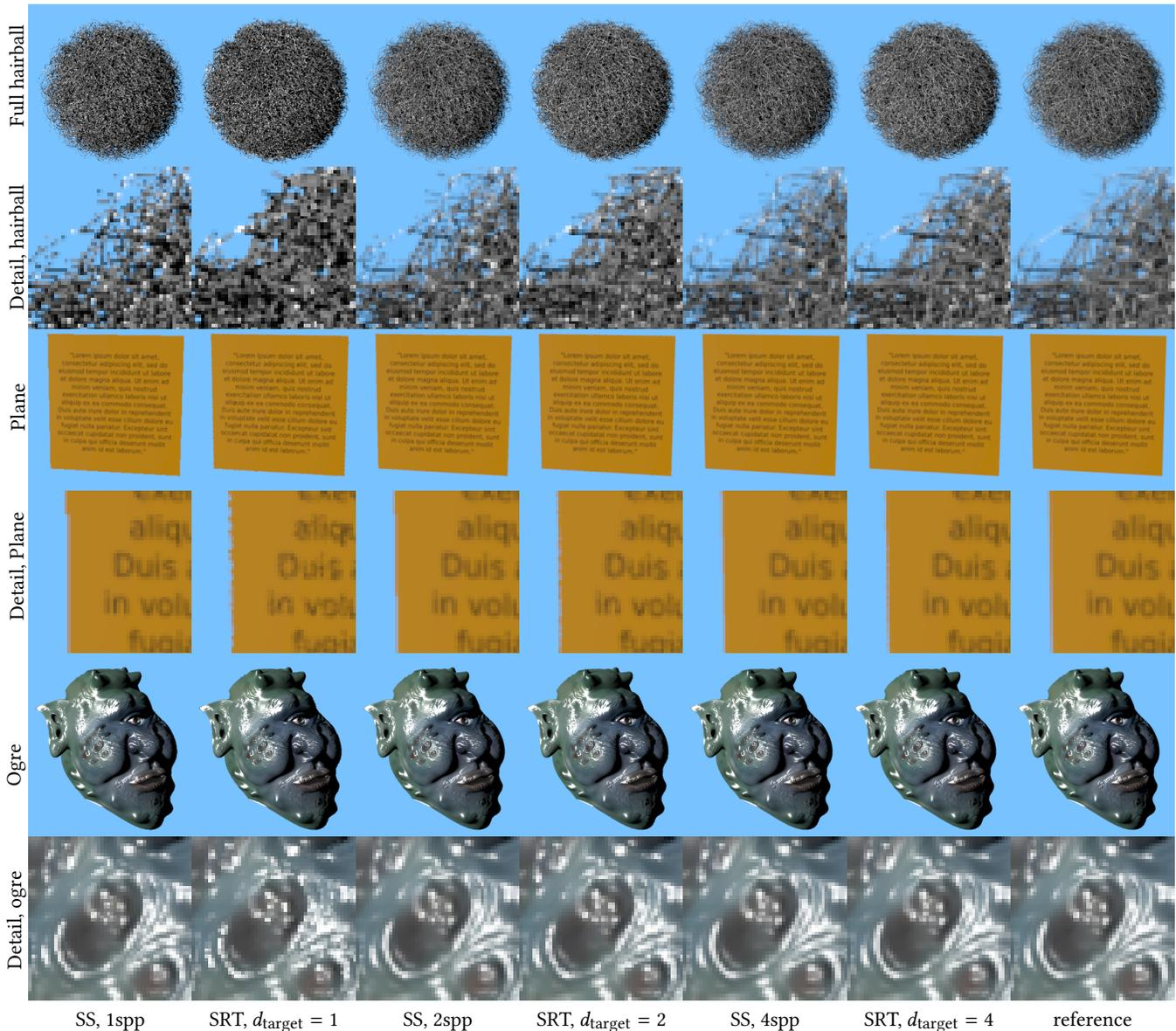
**Figure 8: Quality comparisons between standard supersampling (SS) and stable ray tracing (SRT), for different number of samples. We use the same Gaussian reconstruction filter for all images. For low sample counts, stable ray tracing gives a result that is more temporally stable, at the price of introducing spatial aliasing artifacts.**
