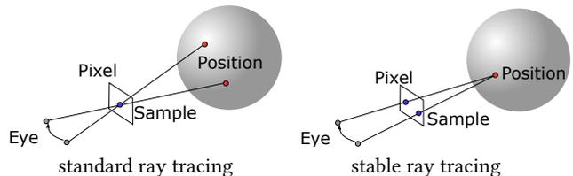
**Figure 1: In standard ray tracing, sampled screen space locations are kept fixed and shading locations vary. In stable ray tracing, shading locations are kept static while screen space locations vary.**
