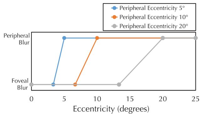
Fig. 3. We use the above foveation mappings for our user studies. For each peripheral blur (5°, 10°, and 20°), we linearly increase the foveation blur radius from 0 to the maximum in a transition region whose width is 33% of the far-peripheral eccentricity. We vary the maximum/peripheral blur in our experiment to compute perceptual thresholds.
