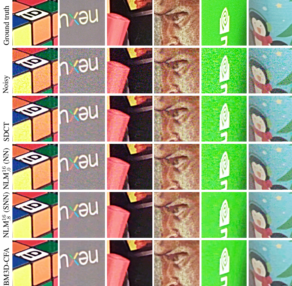
Figure 6: Comparison of several patches from the image on the top, acquired with and NVIDIA Shield Tablet at ISO 1200, demosaiced and then denoised with the different algorithms. Color correction, white balancing, gamma correction and unsharp masking have also been applied after denoising. The ground truth image is obtained by averaging 650 frames. Better seen at 400% zoom.
