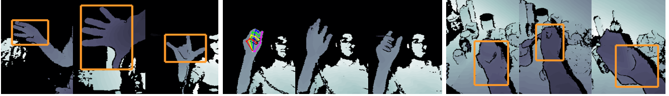
Figure 1: Evaluated tasks. For each scenario the goal is to infer the 3D locations of the 21 hand joints from a depth image. In Single frame pose estimation (left) and the Interaction task (right), each frame is annotated with a bounding box. In the Tracking task (middle), only the first frame of each sequence is fully annotated.
