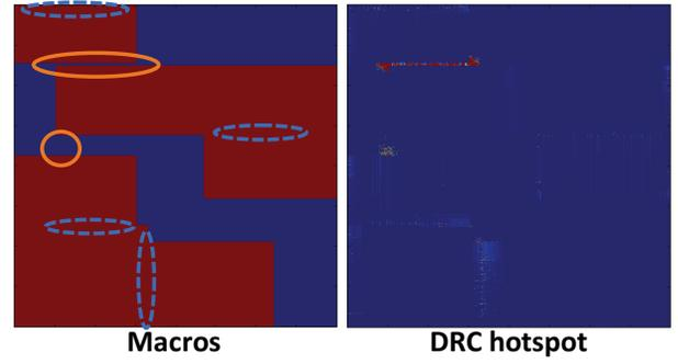
Figure 3: Macros and DRC hotspot distribution. All macros are red rectangles. Orange circles indicate regions with high density of DRC hotspots. Blue dashed circles indicate the remaining sparsely distributed hotspots.
