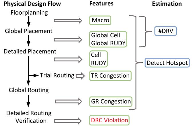
Figure 5: Feature extraction in physical design flow.
