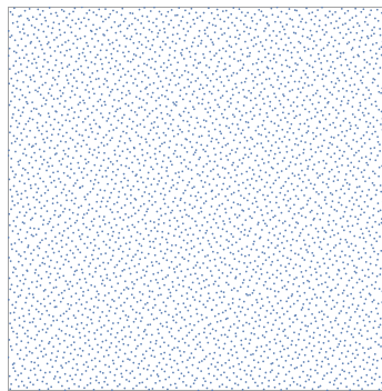
Figure 1. 4,096 pmj02bn samples generated using our technique. These points are progressive, satisfy all applicable power-of-two elementary intervals, and have optimized spectral properties. They were generated in 5.19 ms on a single core of a 4 GHz CPU.
