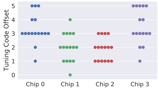
Fig. 11. Variation in replica path tracking across four different chips. Each data point represents the best achievable tuning code for one partition.
