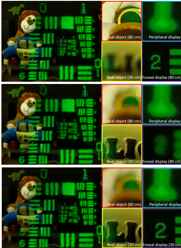
Fig. 16. Focus changing experiment results. A police car, lion doll, and a dinosaur doll are located at the 30, 80, and 250 cm respectively. (top) foveal display plane: 80 cm and camera focal plane : 80 cm (middle) foveal display plane: 80 cm and camera focal plane: 30 cm (bottom) foveal display plane: 30 cm and camera focal plane: 30 cm.
